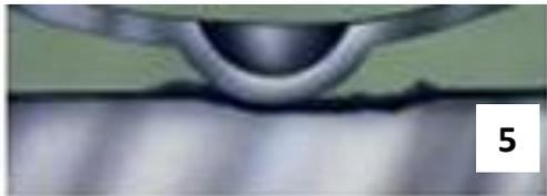
Every time there is motion at the contact spot the cycle repeats and more tin oxide is worn away and debris builds up. (Fig. 5)
