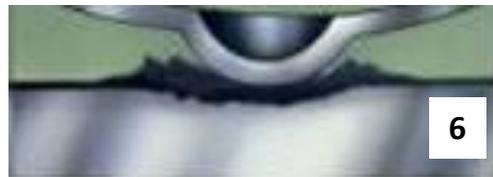
With continued microscopic fretting, enough insulating tin-oxide wear debris can build up high resistance creating intermittent connections. (Fig. 6)
